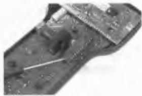
6. The new EPROM chip comes to you with its legs slightly splayed outward. You will need to bend these legs so that they are straight down from the sides of the chip. Place the chip on a flat, hard surface as shown in the diagram and bend the body of the chip so that the legs are straight. Repeat with the opposite side legs.
